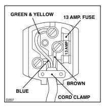
Connect the Green and Yellow (earth) wire to the terminal in the plug which is marked with the letter «E» or the earth symbol
